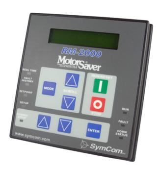
The RM-2000-RTDW motor-monitoring device can be used to monitor and/or control SymCom's Model 777 via an RS-485 Modbus network. Two form C output relays are available for an RTD alarm and a warning alarm. Alarm and trip levels can be set for each RTD to activate the RTD alarm and deactivate the 777 output relay respectively.
